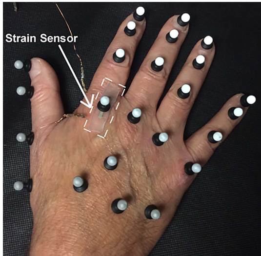
Fig. 2. A strain sensor and reflective markers mounted on the hand of a stroke subject.
