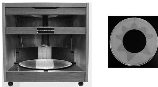
Figure 1 (a) Cusick drapemeter. (b) Configuration of draped image on the Cusick drapemeter.
