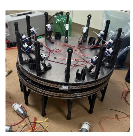
2 disks were cut out using a water jet. Additional holes for wiring were made using a drill press. All other components were mounted to these disks.
