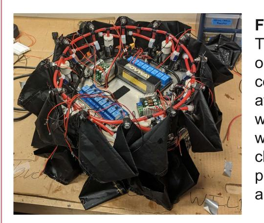
Final Assembly The bladders were bolted on. Electrical components were attached to the aluminum with velcro. The chassis was secured using hose clamps. The rest of the parts were secured using adhesives.
