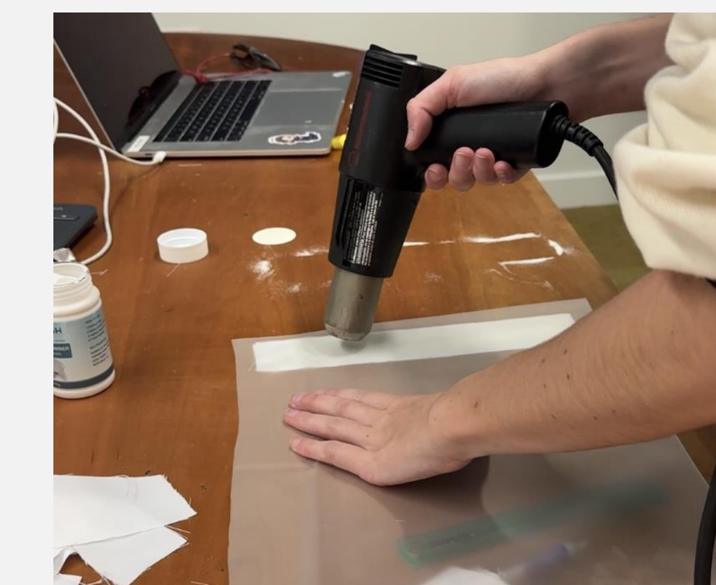
Manufacturing the fabric composite used for FIST's air chambers.
