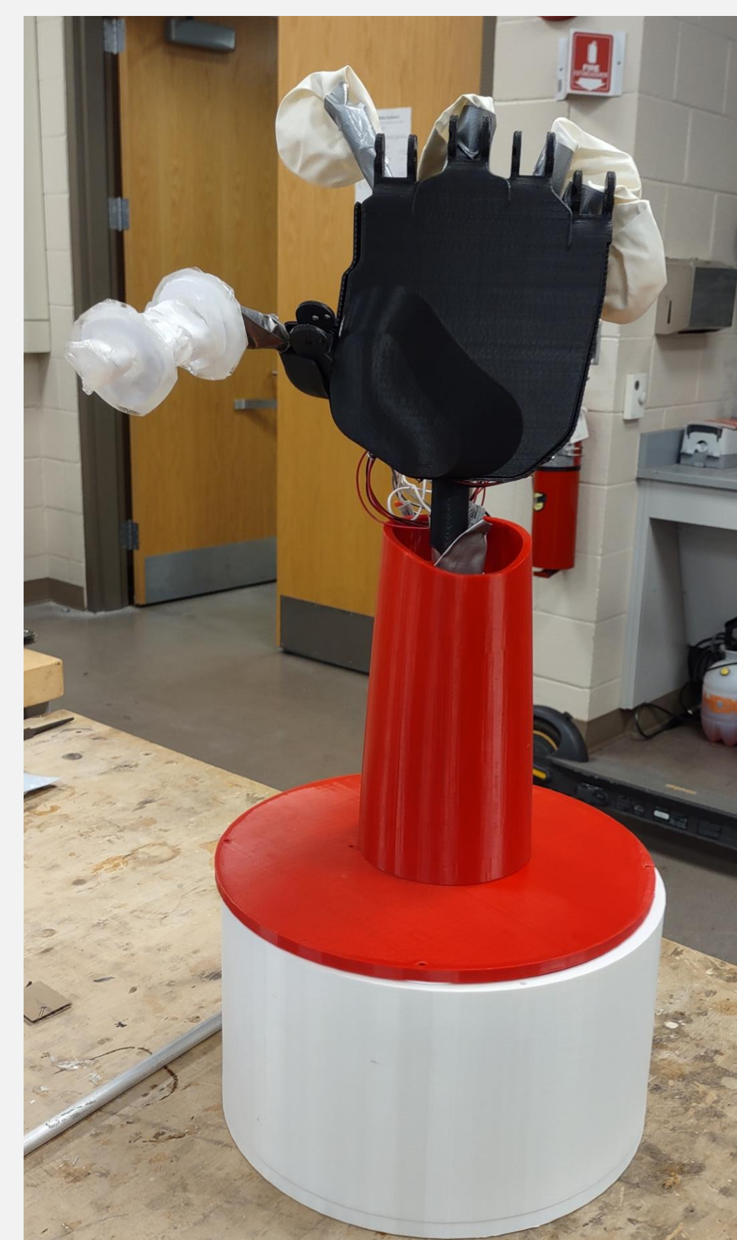
The final prototype of FIST, featuring one of the designed inflatable actuators in the thumb position.
