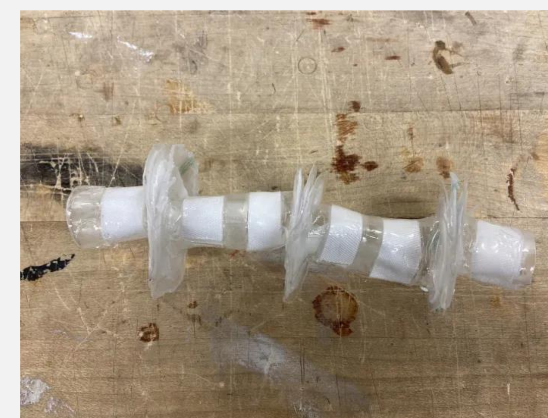
One of the finger designs for FIST. The larger-diameter sections along its length fill with air and expand asymmetrically to create a curling movement.
