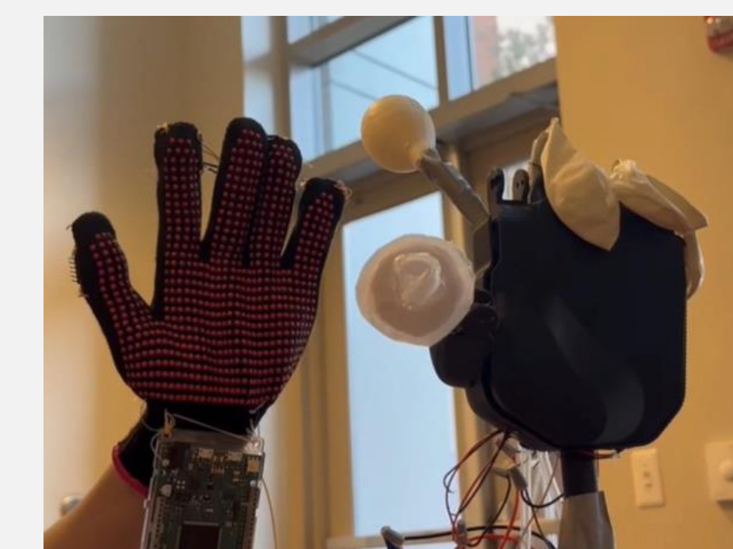
Left: The guidance system which controls the movements of FIST. Right: FIST inflating and deflating several temporary air chambers.
