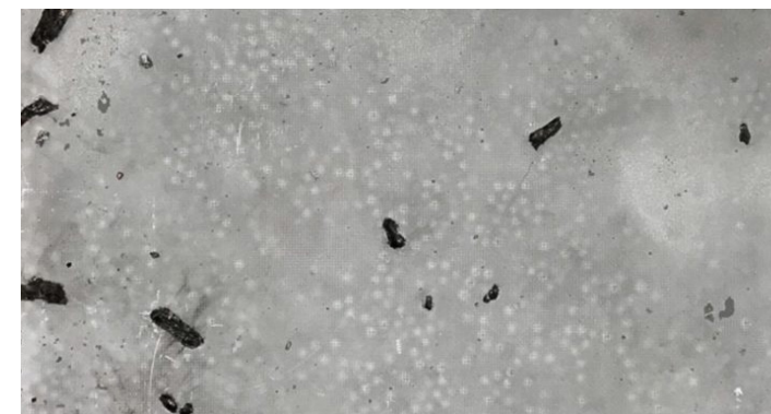
Left: This image shows the CMF panel after the test. The black marks are fragments trapped inside the panel. The image shows there are no cracks or physical bowing -- even after the frags struck at speeds of 5000 feet per second.
