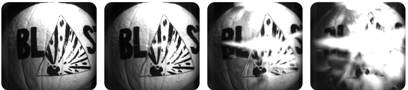
Dynamic fracture of a pumpkin subjected to a simulated bomb blast.
