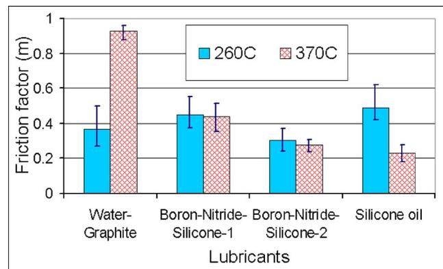
Fig. 9 Influence of temperature on water graphite, boron-nitride-silicone-1, boron-nitride-silicone-2, and silicone oil
