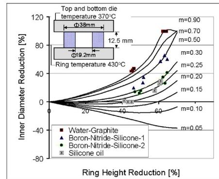
Fig. 8 Friction factors for four lubricants tested at a die temperature of  $370^{\circ}\text{C}$
