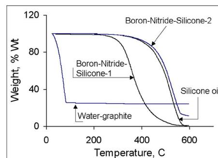
Fig. 3 Thermogravimetric analysis curves of water graphite, silicon oil, boron-nitride-silicone-1, and boron-nitride-silicone-2
