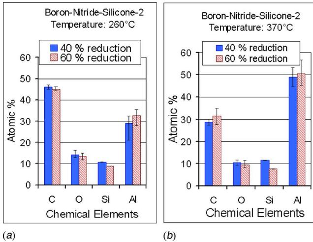
Fig. 13 Lubricant chemical element for boron-nitride-silicone-2 (a) at 260°C and (b) at 370°C
