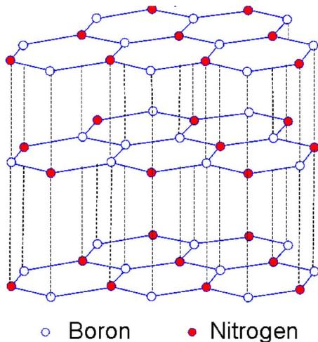
Fig. 1 Structure of hexagonal boron nitride structure
