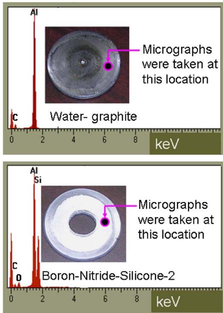
Fig. 10 Spectral analysis and location where micrographs were taken
