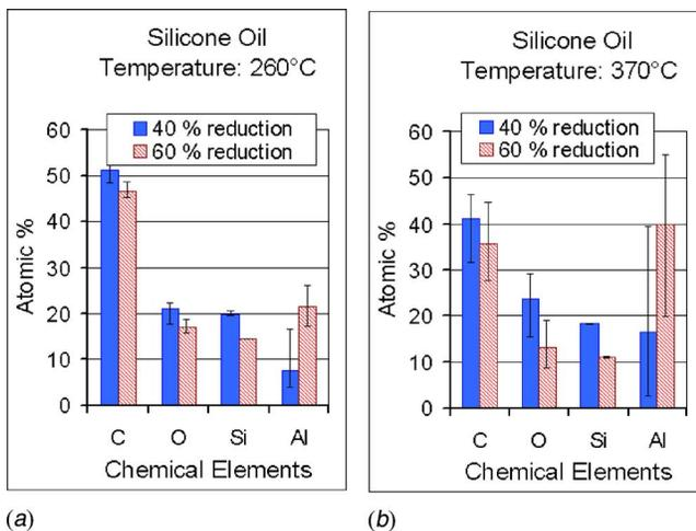
Fig. 14 Lubricant chemical element for silicone oil (a) at 260°C and (b) at 370°C
