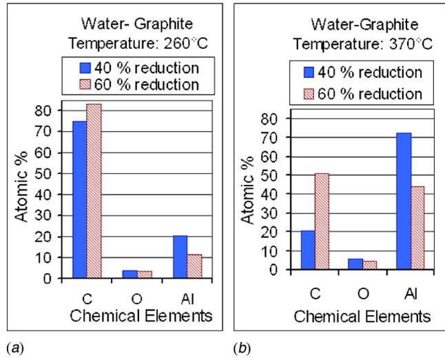
Fig. 12 Lubricant chemical elements for graphite (a) at 260°C and (b) at 370°C
