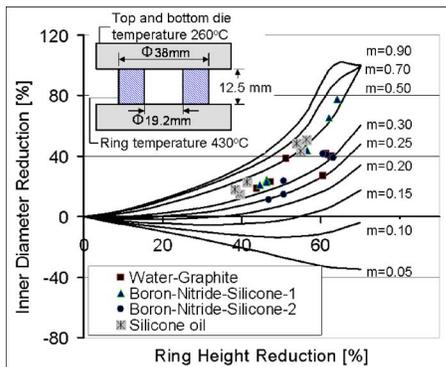
Fig. 7 Friction factors for four lubricants tested at a die temperature of  $260^{\circ}\text{C}$
