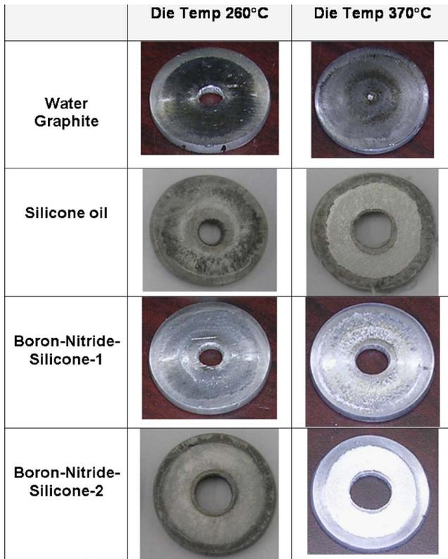
Fig. 6 Deformed samples with graphite, silicone oil, boron-nitride-silicone-1, and boron-nitride-silicone-2 ( $Re=60\%$ )
