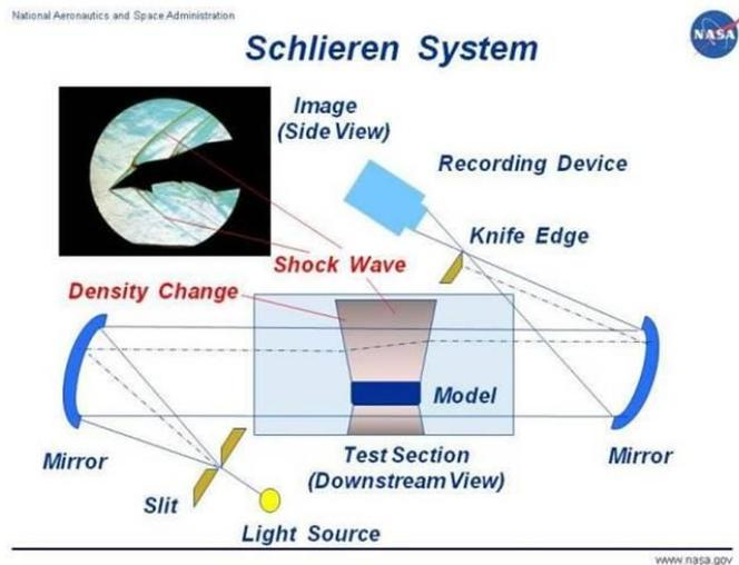
Figure 1: Schlieren system (Source: [www.nasa.gov](http://www.nasa.gov)).
