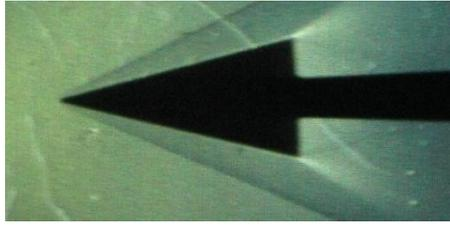
Figure 2: Image of an oblique shock in the NCSU Supersonic Wind Tunnel.
