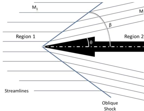
Figure 3: Schematic of an oblique shock.
